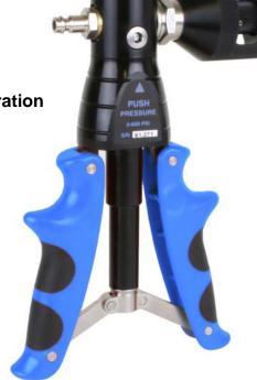
The **7090** is a pressure and vacuum calibration pump that combines performance with rugged design. Its features include contoured cushioned handles for comfort and control, protective caging for the vent valve guarding against accidental damage, and dual o-rings on all pistons to ensure zero leakage.
