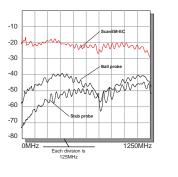
Frequency response of ScanEM-EC vs. passive probes.
