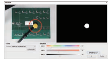
Image recognition (recognized the yellow color at the tip of the probe)
