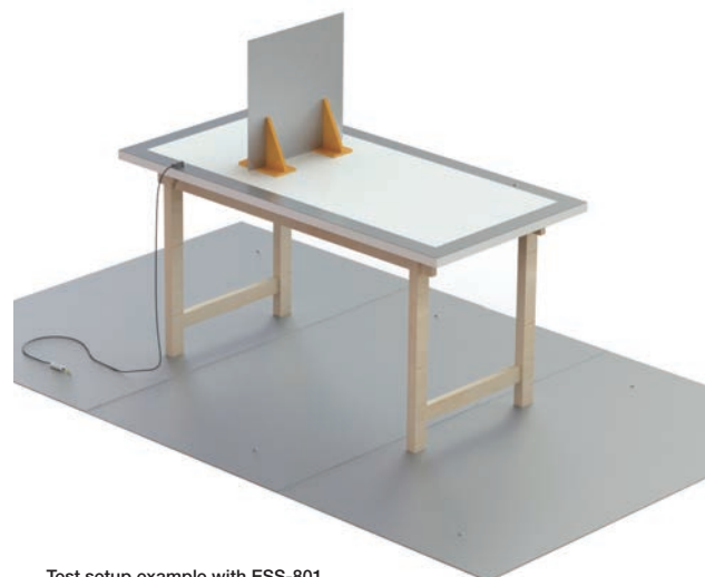
Test setup example with ESS-801 * Contents in the set referred to following specification
