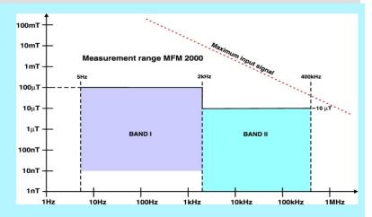
Frequency range: 5 Hz- 2000 Hz (Band I) and 2 kHz- 400 kHz. (Band II)
