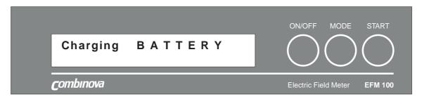
During charging, the battery voltage is constantly checked against different limits by the microprocessor to decide if the charging is working properly.
