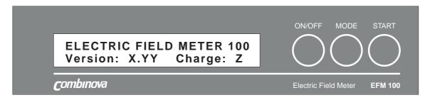
X.YY indicates which software version the instrument is equipped with.
