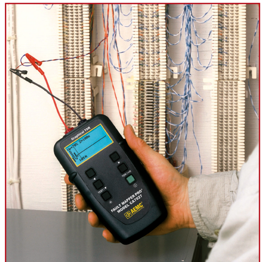
Model CA7027 testing cables in a telephone patch panel.
