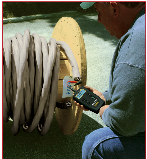
Model CA7024 is used to check length of a power cable on a reel.
