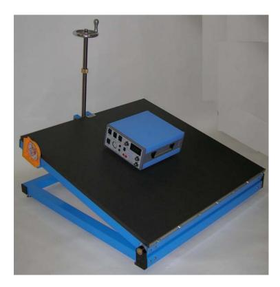
The Inclined Plane Device is used to determine the stability of electric appliances which are used on a table or on the floor.
