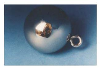
The ED&D Impact Test Balls are high-precisionmachined steel balls, usually chrome plated, used to test impact resistance according to IEC, CSA, CE, EN, MIL, VDE and UL Standards...among others. The units come with removable eyelets, where applicable. The balls come with ISO/IEC 17025 Accredited, in Scope, calibration. NIST-traceable. In stock!
