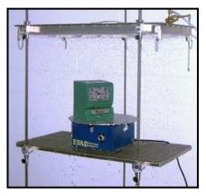
**DESIGN:** Water tank of anodized aluminum with throttling means, including choice of advanced suspension means (wall, ceiling or stand)
